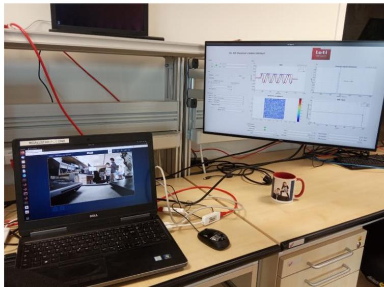
**Figure 16. Validation of over the air uplink. View of the webcam display and of the KPIs GUI.**
