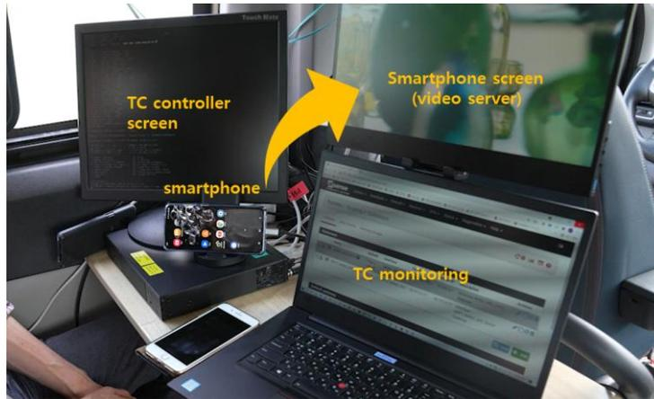
**Figure 32: The video streaming in the vehicle**
