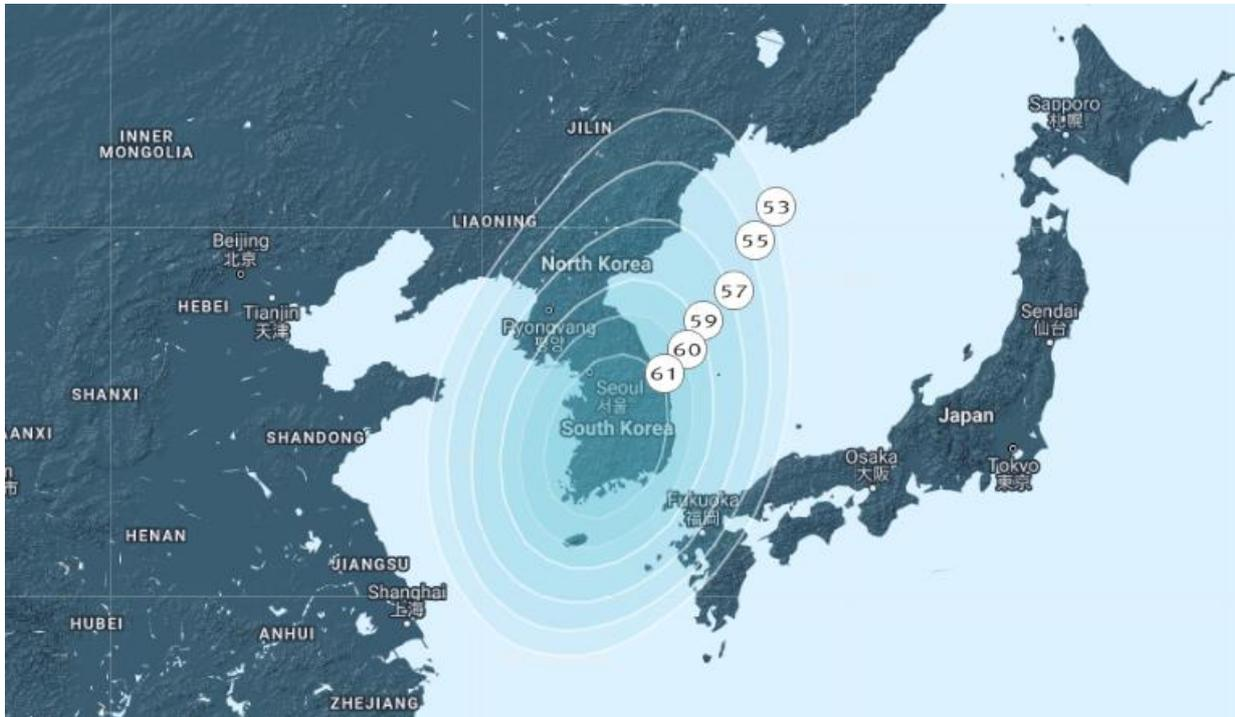
Figure 3-11: Coverage map of KOREASAT 6 (EIRP of FSS Ku-band beam).
