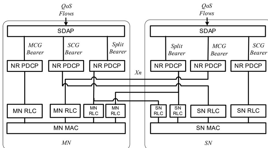
Figure 4-1: Network side protocol termination options for MCG, SCG and split bearers in MR-DC with 5GC [14].
