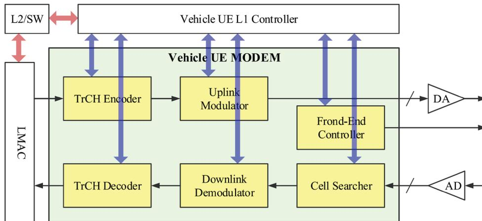
Figure 6-4: Architecture and interface of V-UE modem.
