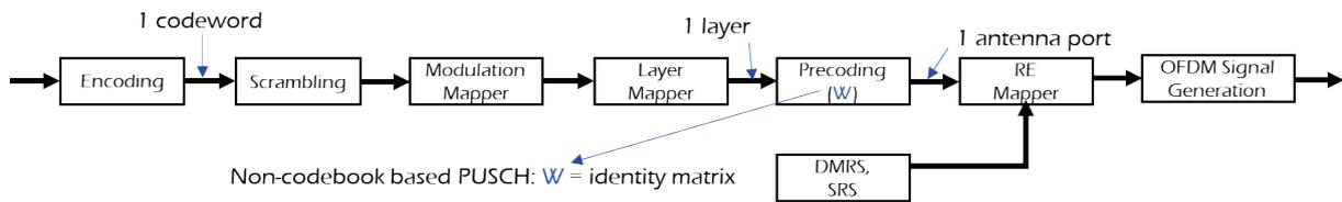
Figure 5-2: Uplink baseband processing.
