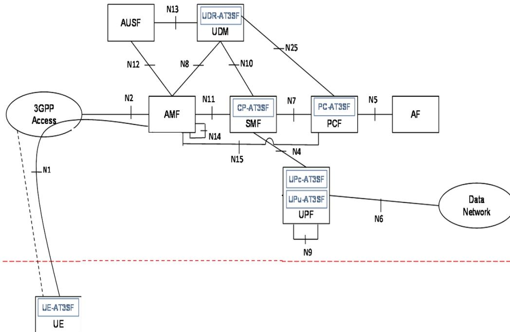
**Figure 9-1: 3GPP AT3SF / ATSSS architecture (3GPP access only).**
