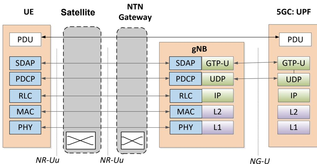
**Figure 3-14: UE control plane protocol stack for a PDU session (transparent satellite).**
