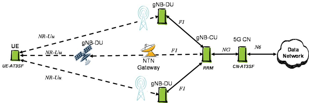
Figure 4-9: Architecture of MC7.
