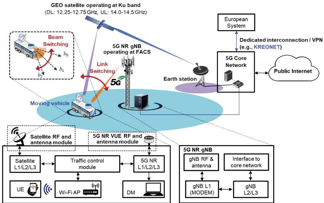
**Figure 6-2: Overall architecture and interface for Korean access system.**
