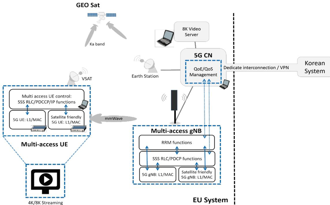
**Figure 6-1: Overview of the EU system and interfaces between the different sub-modules.**
