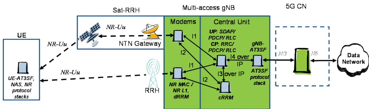
Figure 4-5: Architecture of MC3 (preliminary architecture for EU MC PoC).
