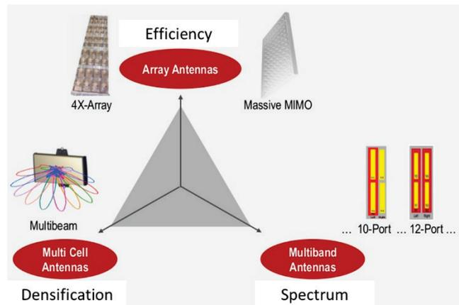
**Figure 3-12: From [13]. Magic triangle for antennas.**
