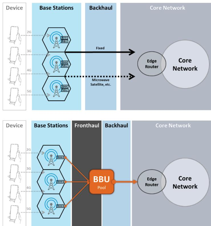
Figure 3-11: From [12]. Top: overview of a mobile network. Bottom: C-RAN architecture.
