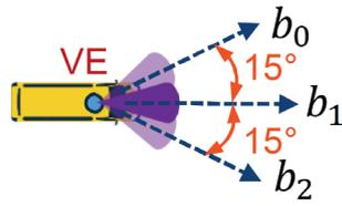
Figure 5-8: An example of beam switching with three available beams.
