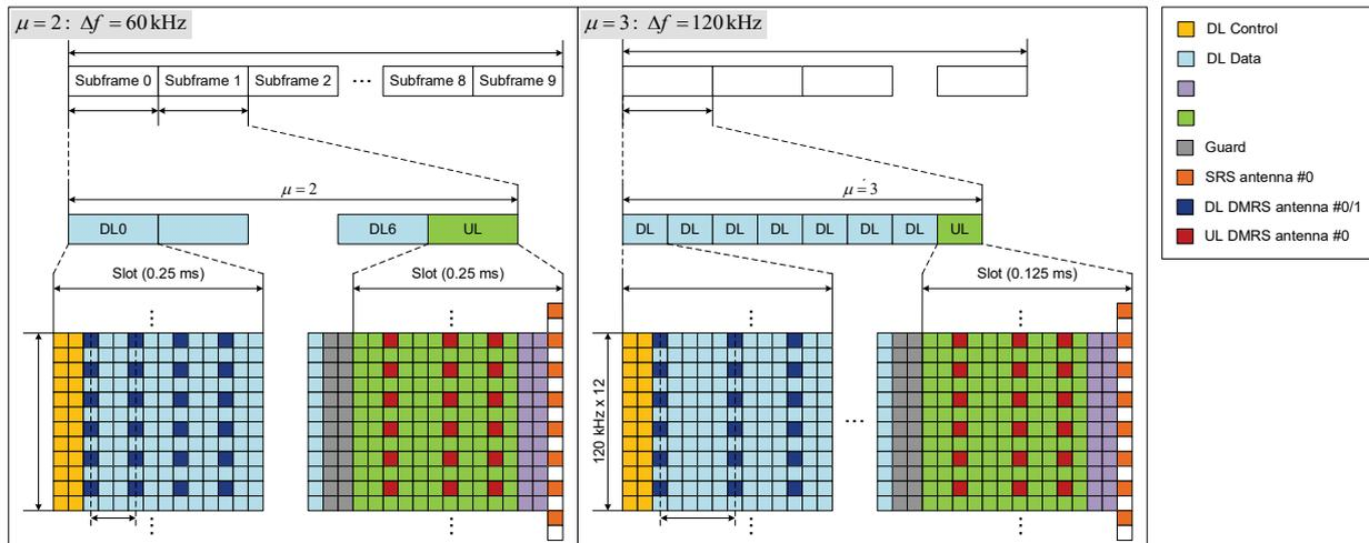
Figure 5-7: Frame structure (numerology and DMRS pattern).
