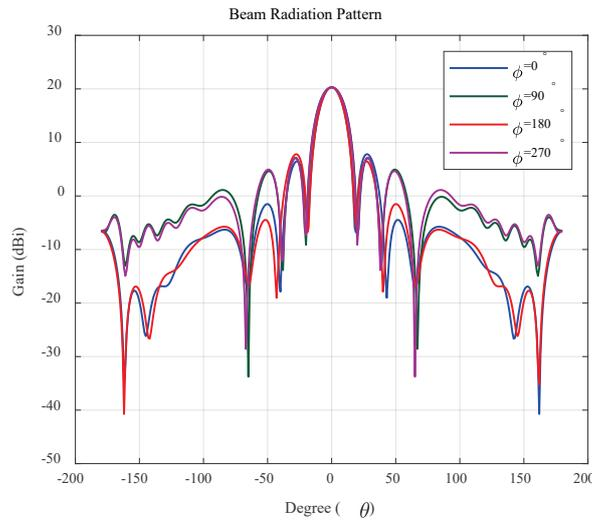
Figure 5-4: Target beam radiation pattern of each antenna panel.
