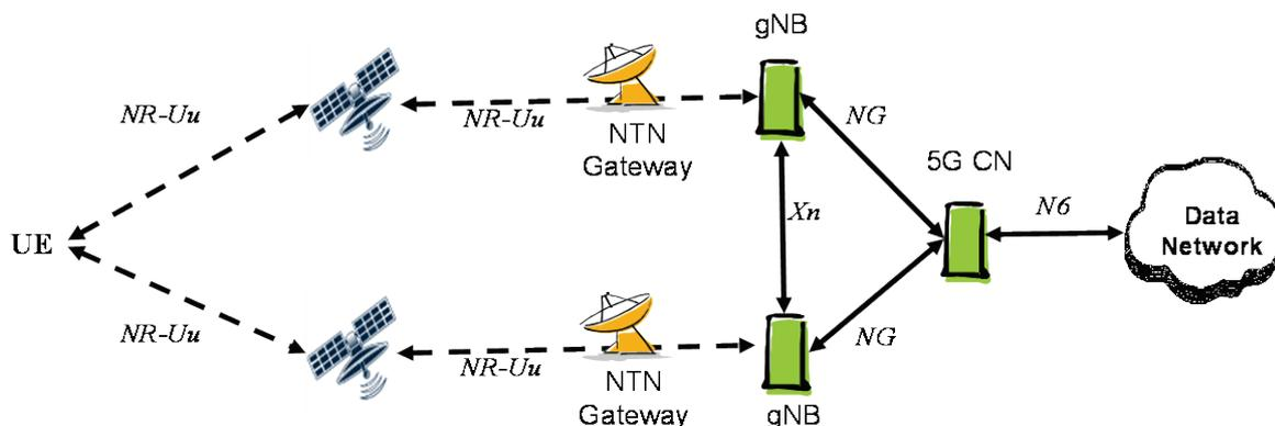
**Figure 4-6: Architecture of MC4.**
