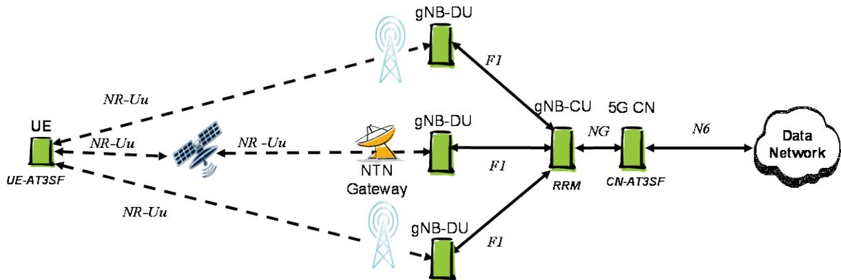
**Figure 4-4: Architecture of MC2.**
