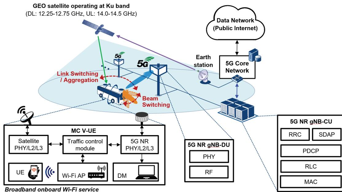
**Figure 4-12: Architecture of MC10 (preliminary architecture for KR MC PoC).**
