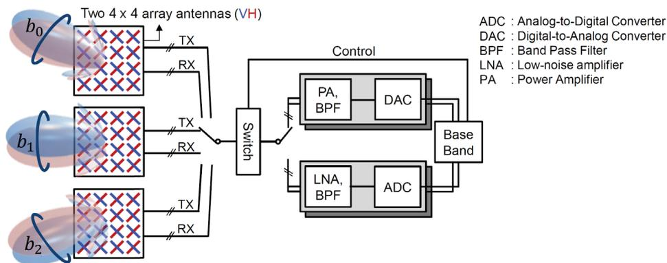
Figure 5-3: Basic idea of antenna and RF module design for beam switching at V-UE.
